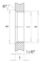
Installation direction: o-ring sits on chamfer.
